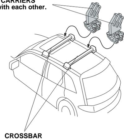
8. Turn the knobs on the top clamp to tighten the front carrier.
