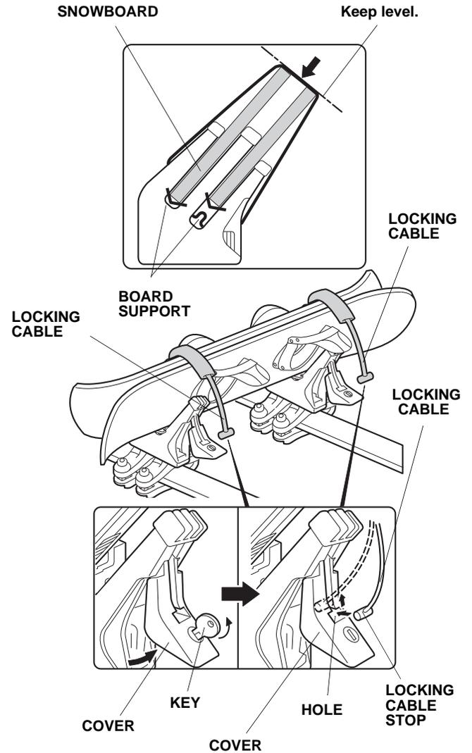
16. Check that the locking cables are installed securely, then close the covers.
